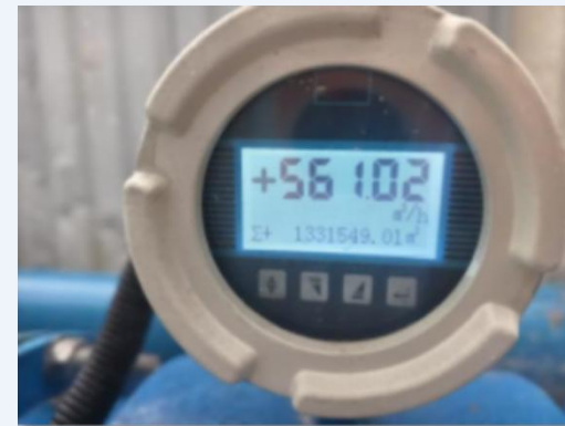
Installation of flow meters at the inlet and outlet, and online monitoring systems at the mine water treatment station
