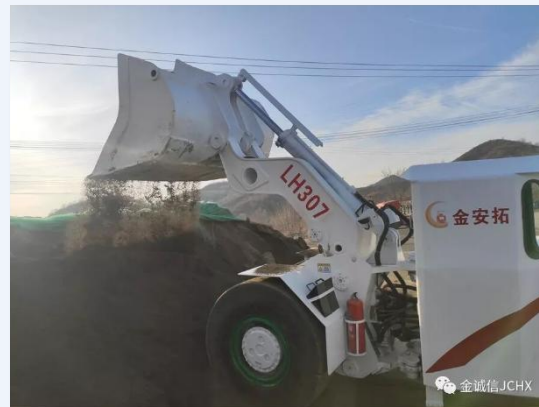
Self-developed electric LHD featuring low noise and zero emissions
